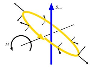
Figure 13.16: Electric motor using a single wire loop. The Lorentz forces (black vectors) exerted by the external magnetic field on the electric current carriers in the wire produce a net moment M on the loop. The self-induced magnetic field of the wire and the corresponding radial forces are not shown.
