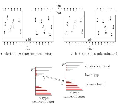
Figure 6.37: Peltier cooling. Top: physical device. Bottom: Electron energy spectra of the semiconductor materials. Quantum states filled with electrons are shown in red.
