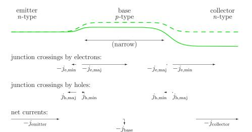
Figure 6.35: Schematic of the operation of an n-p-n transistor.
