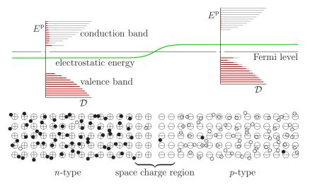
Figure 6.33: The p-n junction in thermal equilibrium. Top: energy spectra. Quantum states with electrons in them are in red. The mean electrostatic energy of the electrons is in green. Below: Physical schematic of the junction. The dots are conduction electrons and the small circles holes. The encircled plus signs are donor atoms, and the encircled minus signs acceptor atoms. (Donors and acceptors are not as regularly distributed, nor as densely, as this greatly simplified schematic suggests.)
