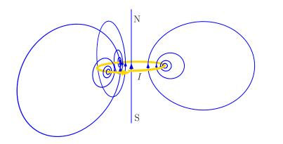
Figure 13.14: An electromagnet consisting of a single wire loop. The generated magnetic field lines are in blue.
