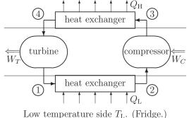
Figure D.4: Schematic of the Carnot refrigeration cycle.
